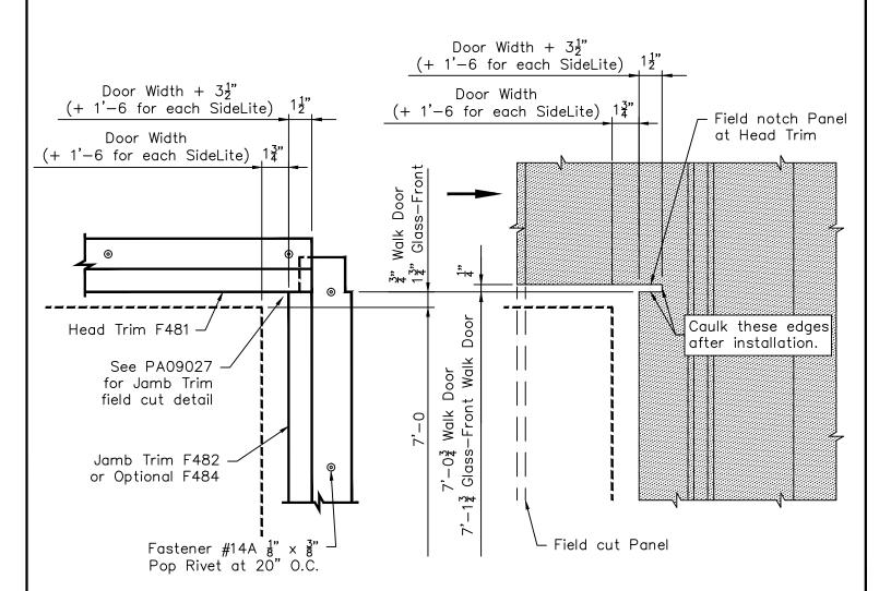
Note: All trim is to be installed BEFORE blanket insulation is applied to walls
